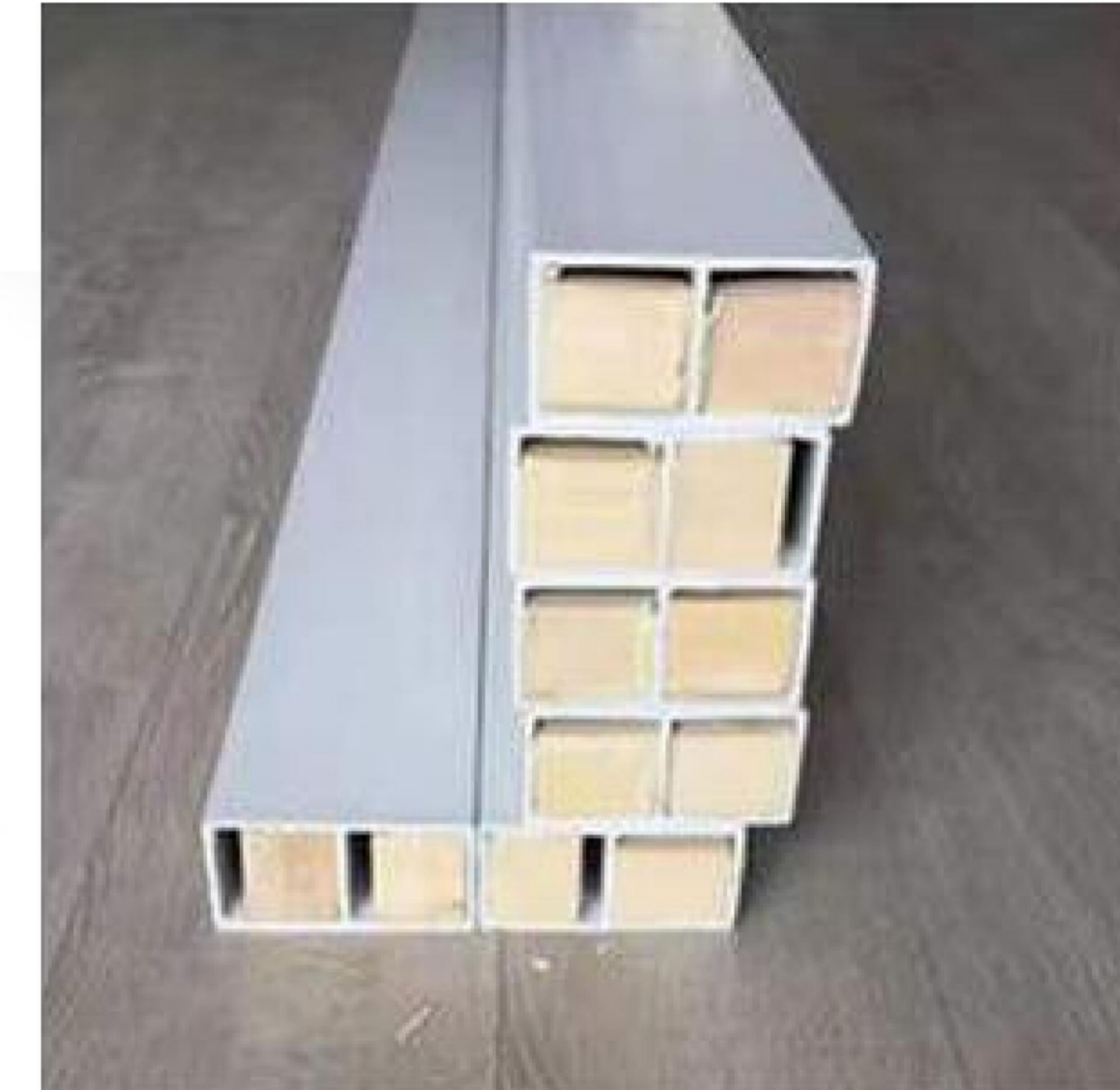
2. Fix the bottom of the timbers by putting the wood blocks in the timbers and then fixing the blocks and timber together by nail-free adhesive.
